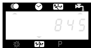
845 litres of treated water remaining
