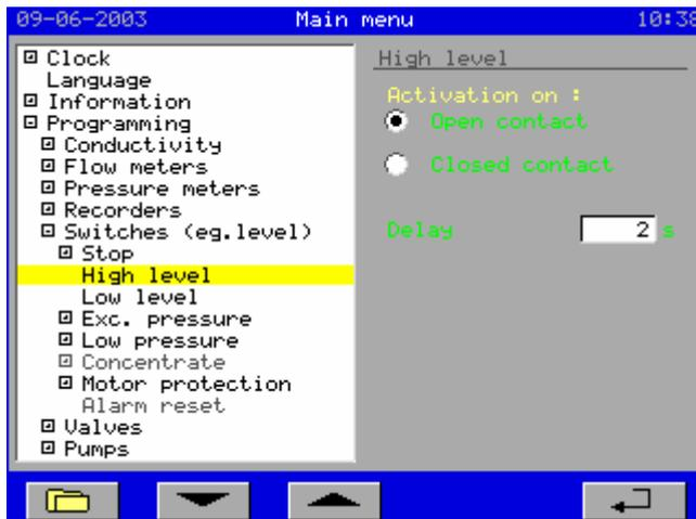
In this window, you must set the properties for the “high level” switch in the storage tank.
