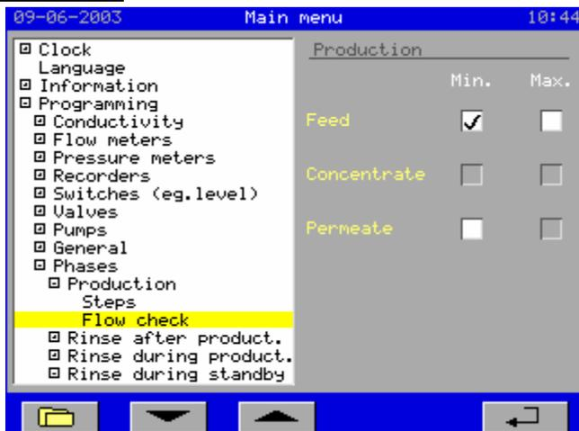
In the **“Programming - Flow meters”** options (§ 9.3 “Flow measurement” 23), the monitoring must be activated for a flow measurement.
