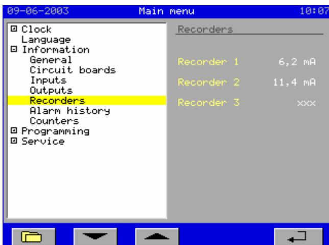
This window displays the status of the power (recorder) outputs, if the optional recorder PCB has been installed.
