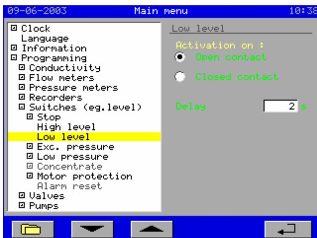
In this window, you must set the properties for the “low level” switch in the storage tank.
