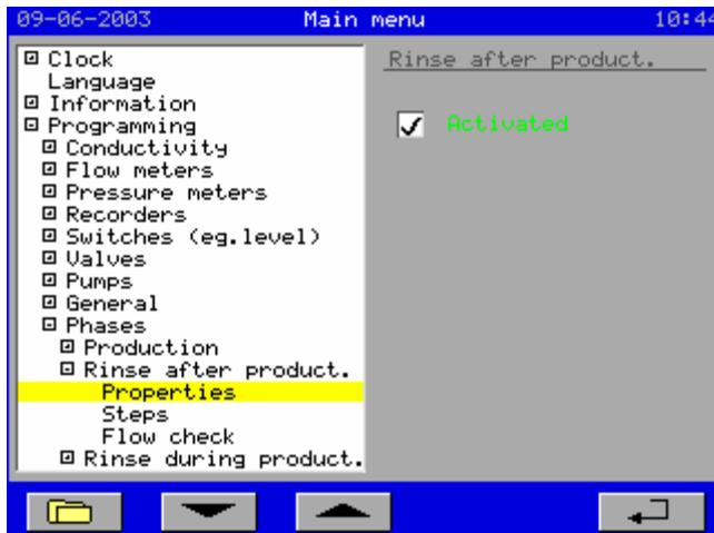
You can set whether a membrane rinse will occur after the production of desalinated water has stopped.
