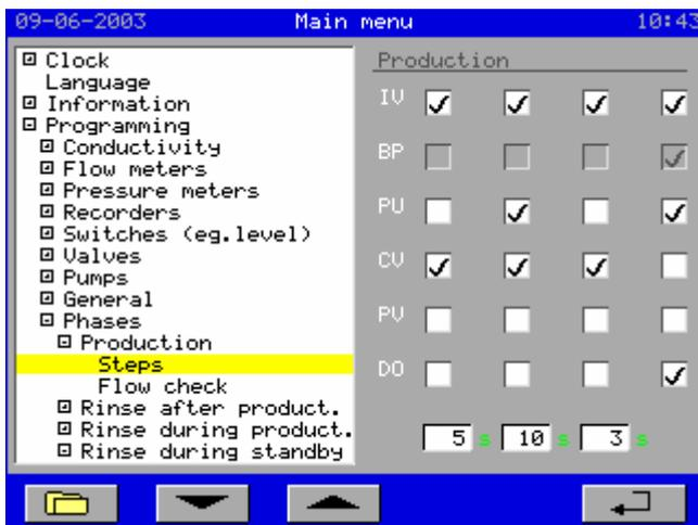
In this window, you can set the output functions to be activated for each “sub”-phase.
