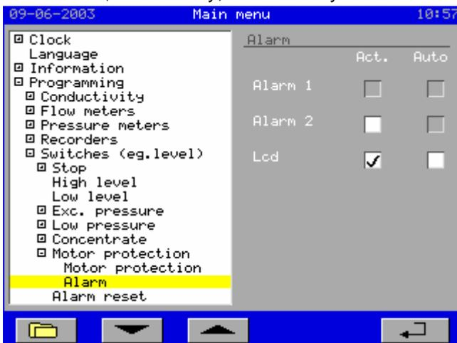
In the programming of a particular malfunction, you can indicate whether the system must be switched off and whether the system will switch back on automatically once the malfunction is removed.
