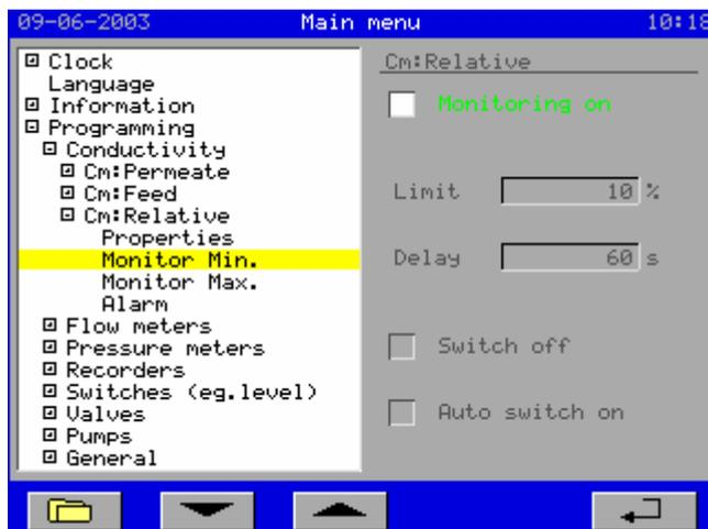
In this window, you can activate the monitoring of the minimum relative conductivity.
