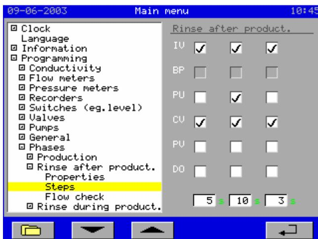
In this window, you can set the output functions to be activated for each “sub”-phase. The duration of the three start-up phases can be given.
