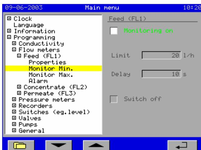
In this window, you can activate the monitoring of the minimum flow.
