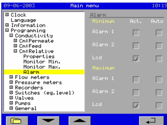
In this window, you can set whether a message should appear in the “alarm window” (“**LCD**” Act. option) and whether an alarm output should be activated in the event of a faulty measurement value.
