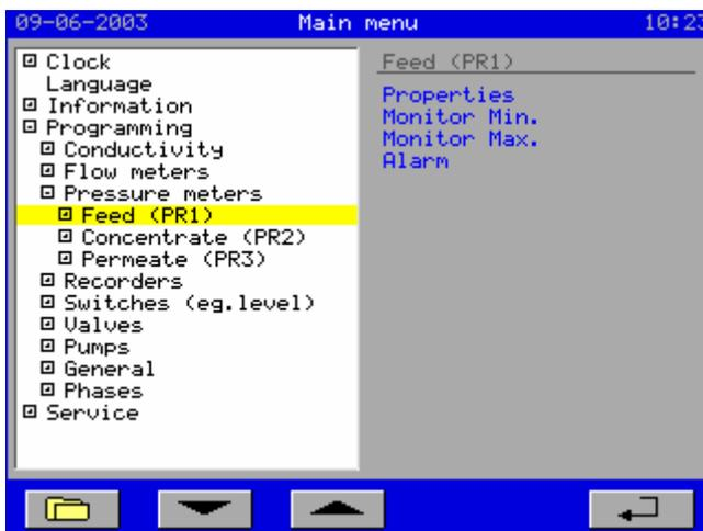
The settings for the pressure meters are located inside the “**Programming – Pressure meters**” folder. This folder is subdivided into the pressure measurement for the feed, the concentrate and the permeate.
