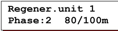
During regeneration, the second line of the LCD display shows the remaining time for the current phase and after the oblique the remaining time for the whole regeneration.
