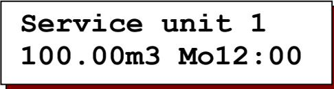
The first line of the LCD display shows the present state of the system, e.g. "Filter1 in service", "Filter 2 in regeneration" or "not in service".
