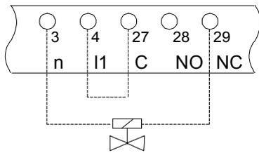
Connection to a magnetic valve active when voltage not applied on potential free relay output :
