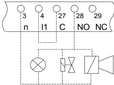
Connection to a signal lamp, klaxon or magnetic valve active when voltage applied on potential free relay output :
